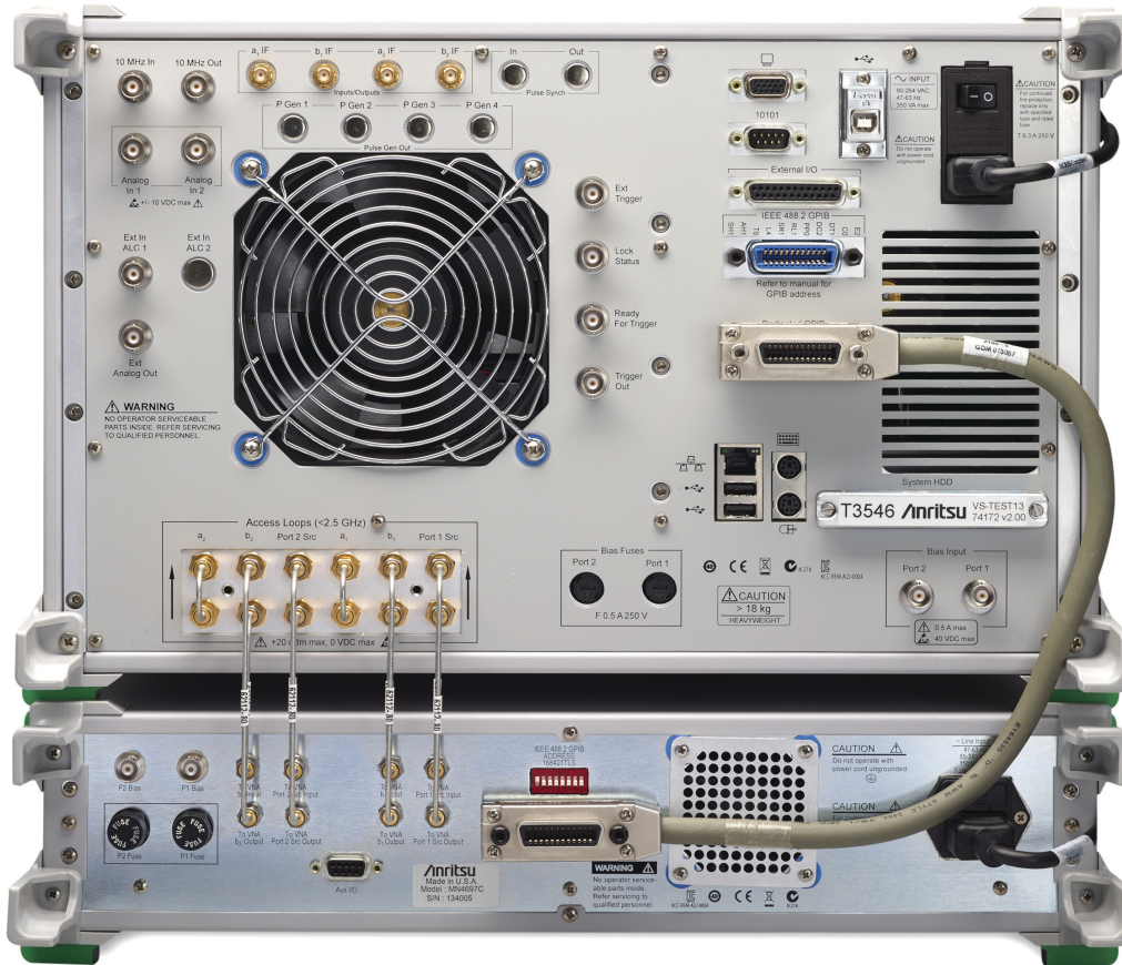
MN469xC Test Set Rear Panel and Connections to Base VNA
